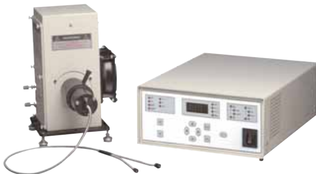
96000 150 W Solar Simulator with Bifurcated Bundle.
